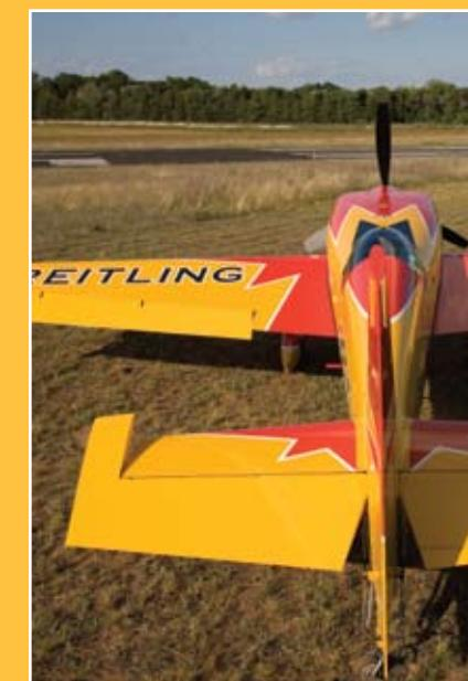
From nose to tail, the new Extra 330SC incorporates changes that make it lighter and more maneuverable. Mechanically adjustable foot pedals and carbon fiber push rods save weight, while trapezoidal ailerons and new geometry on the tail improve rolling and tumbling maneuvers.
