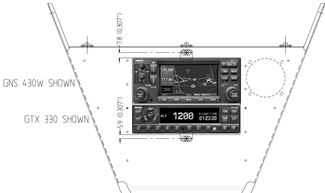
Figure 6: Position of safety clamps (EA 300/L shown)
