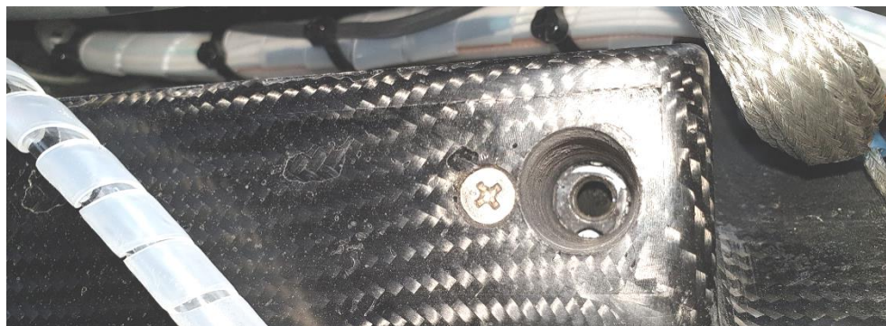
Fig. 14 – Diameter of hole increased to 17 mm all the way up to the nutplate
