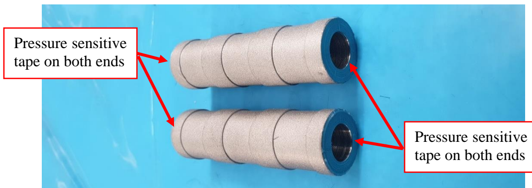
Fig. 15 – Prepared bushings (sandblasted)
