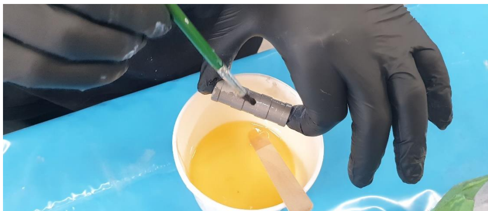
Fig. 19 – Application of epoxy-resin to the cylindrical surface of the bushing
