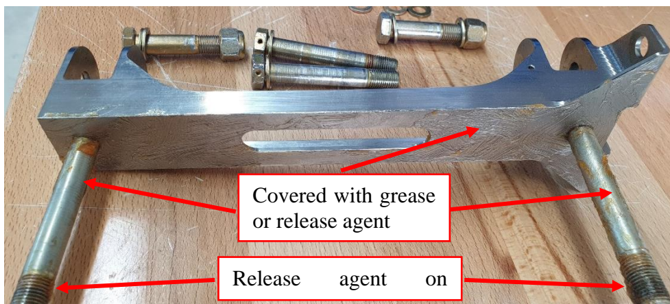
Fig. 16 – Fuselage mounting bracket prepared with release agent / grease
