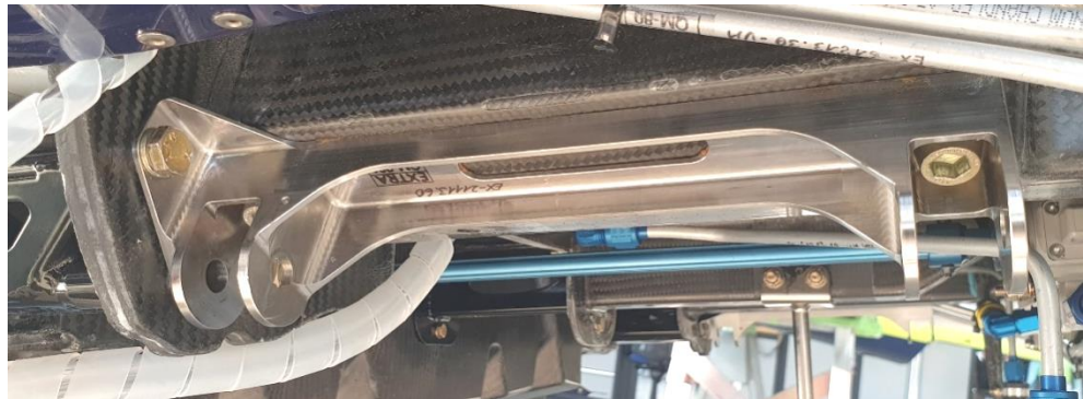
Fig. 26 – Bracket completely reinstalled and all bolts torqued
