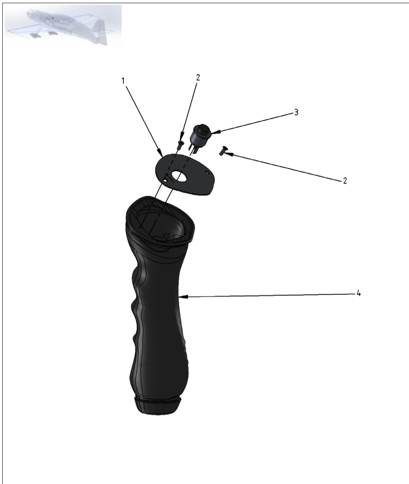
Figure 27-9 Copilot Control Stick Cover
